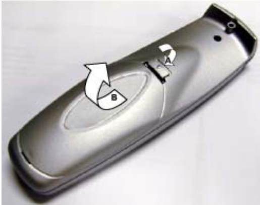
Image 2-5 Battery cover unlock
